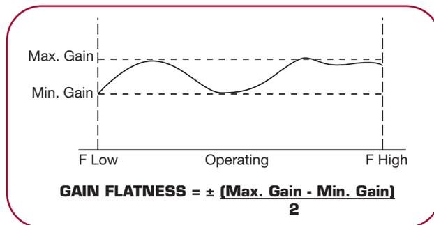
Test data supplied with our amplifiers will include swept gain plots taken at least 100 to 1600 points within the band. Tabular data can also be supplied if required.
