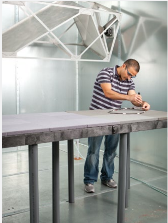
Mode stir RF-Shielding testing per IEC Standard 61000-4-21 Annex F
